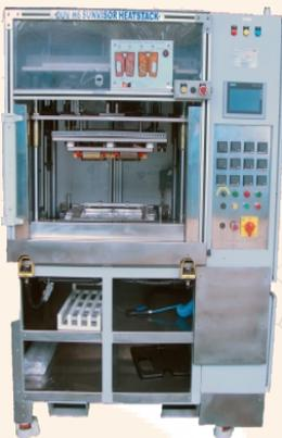
Sun Visor Heat Stack Welding Machine
